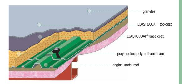
The ELASTOSPRAY<sup>®</sup> spray-applied polyurethane foam (SPF) roofing system from BASF Polyurethane Foam Enterprises LLC delivers a cost-effective and sustainable solution for aged and leaking metal roofs – one that economically provides new life to the existing metal roof.
