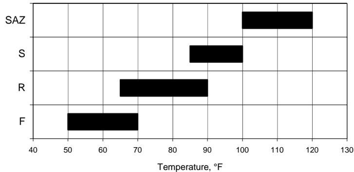
The temperature ranges pictured above are meant as general suggestions only. Ultimately, the experience of the applicator should determine which reactivity grade is best suited for any specific combination of substrate (composition, location, color, etc.) and ambient conditions. Please contact your BASF Polyurethane Foam Enterprises LLC representative with any questions or for more specific assistance.
